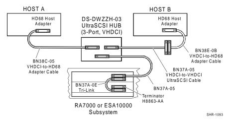
NOTE: In hub configurations, termination is internal to the hub.
